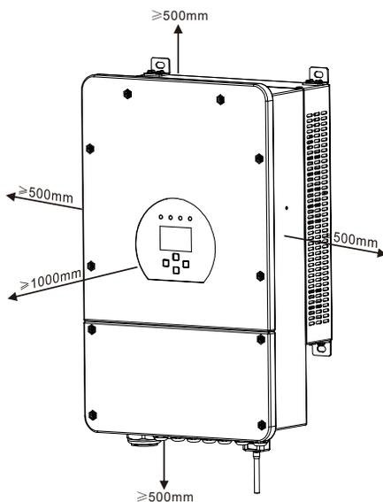
For proper air circulation to dissipate heat, allow a clearance of approx. 50cm to the side and approx. 50cm above and below the unit. And 100cm to the front.
