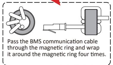
Pass the BMS communication cable through the magnetic ring and wrap it around the magnetic ring four times.
