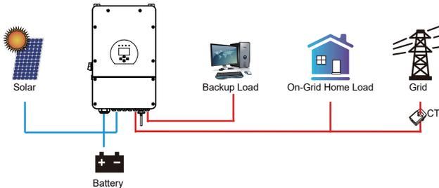
**Solar Sell:** “Solar sell” is for Zero export to load or Zero export to CT: when this item is active, the surplus energy can be sold back to grid. When it is active, PV Power source priority usage is as follows: load consumption and charge battery and feed into grid.
