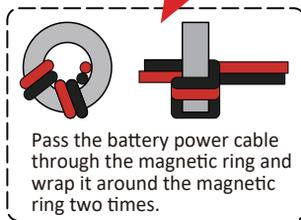
Pass the battery power cable through the magnetic ring and wrap it around the magnetic ring two times.
