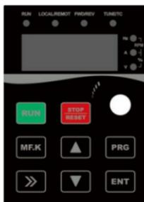
The controller has a total of three levels of menus, which are: ① Parameter team (first level menu); ② Parameter number (second level menu); ③ Parameter set value (level 3 menu). Taking setting the power-on automatic start function FD.11=1 as an example, the following flow chart of adjusting parameters is listed:
