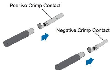
**Step 3** Insert the crimped cables into the corresponding connectors until they snap into place. Gently pull the cable backward to ensure firm connection.
