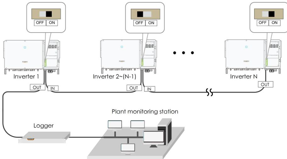
Figure 5-5 Configuration of dip switch ( $N \geq 15$ )
