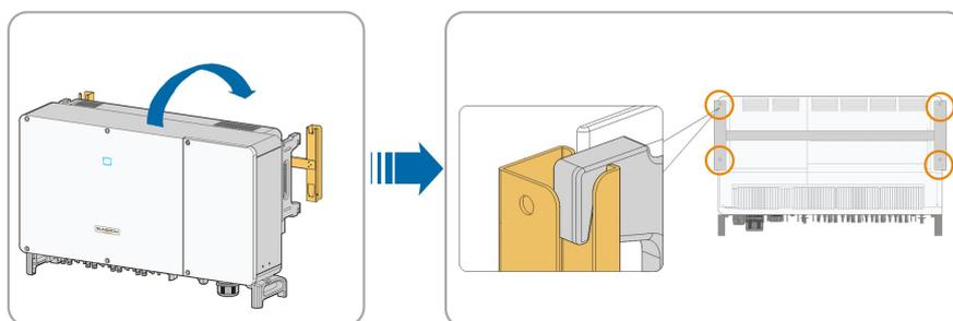
**Step 8** Fix the inverter with screws.
