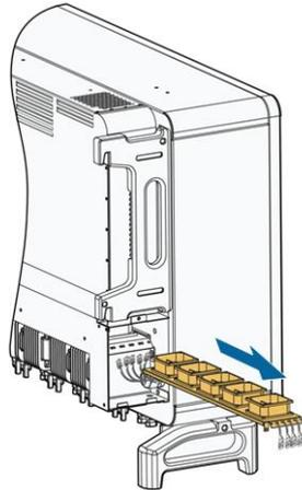
**Step 5** Follow the steps above to remove the fan on the other side of the inverter.
