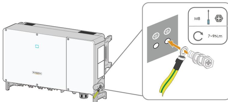
**Step 3** Apply paint to the grounding terminal to ensure corrosion resistance.
