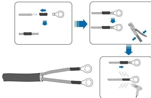
**Step 6** Stack the OT terminals on the OT/DT terminal of the AC cables, and fix the cables to corresponding terminals.
