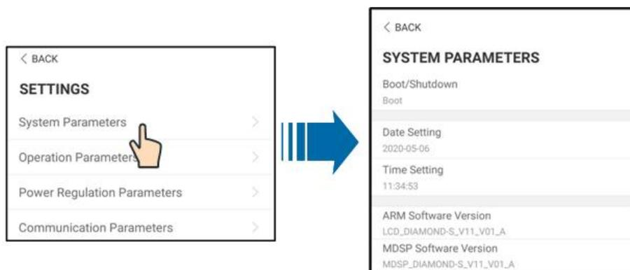
Figure 7-13 System Parameters
