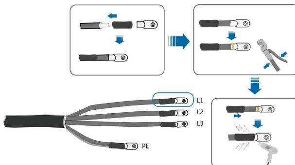
**Step 8** Secure the wires to corresponding terminals.
