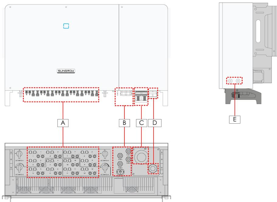
Figure 5-1 Wiring terminals
