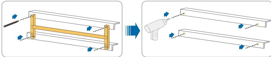
**Step 3** Secure the mounting-bracket with bolts.
