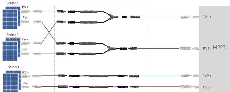
**Case 2 :** When the Y terminal is connected at the inverter side, the Y terminal can be directly connected to the DC side of the inverter, and the system wiring diagram is shown in the figure below.
