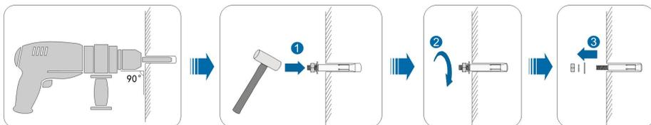
**Step 4** Fix the mounting-bracket with the expansion bolts.
