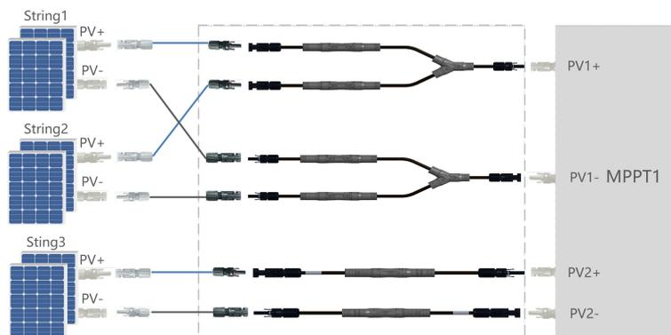
Sungrow can provide Bizlink's Y-branch connector. If necessary, please contact Sungrow to purchase. Customers can also purchase Y-branch connector of the same specification by themselves. The wiring instructions for Y-branch connector are as follows.
