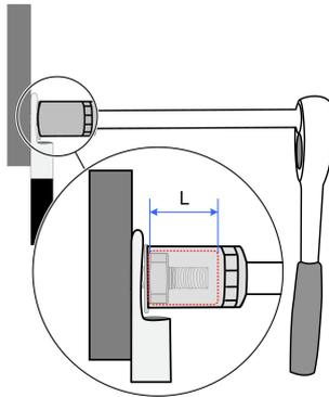
**Step 9** Gently pull the cable backwards to ensure firm connection, and fasten the swivel nut clockwise.
