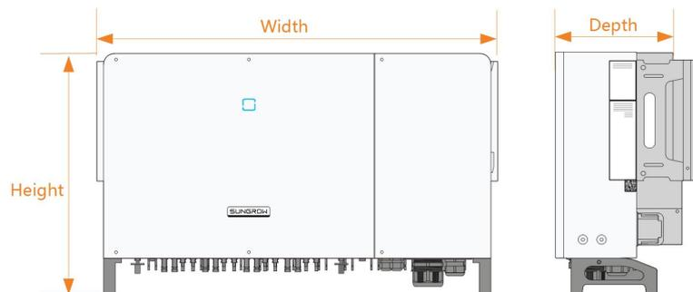
Figure 2-2 Dimensions of the Inverter
