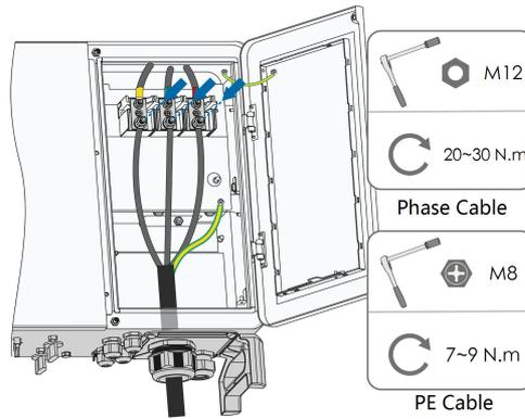
Ensure that the depth L of the socket used is not less than 28mm.
