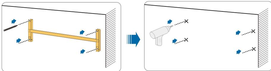
**Step 3** Insert the expansion bolts into the holes and secure them with a rubber hammer. Fasten the nut with a wrench to expand the bolt. Remove the nut, spring washer, and flat washer, and store them properly.
