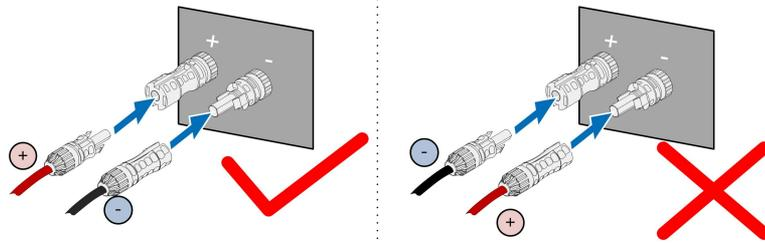
Arc or contactor over temperature may occur if the PV connectors are not firmly in place, and SUNGROW shall not be held liable for any damage caused.
