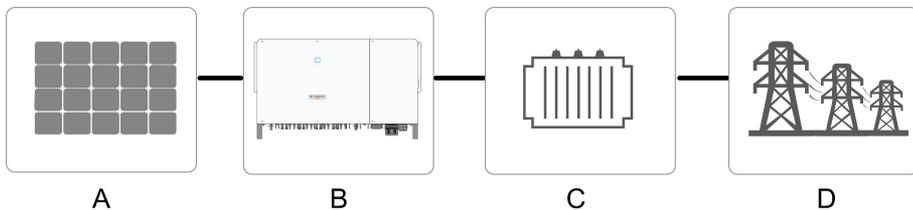
Figure 2-1 Inverter application in PV power system
