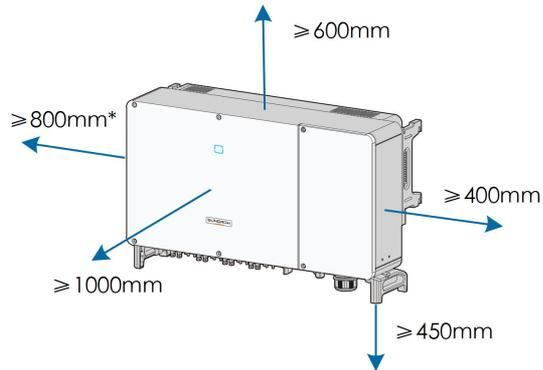
\* The distance can be shortened to 200mm according to onsite conditions. In case the distance is less than 800mm, move the inverter from the mounting-bracket or wall before maintaining fans.
