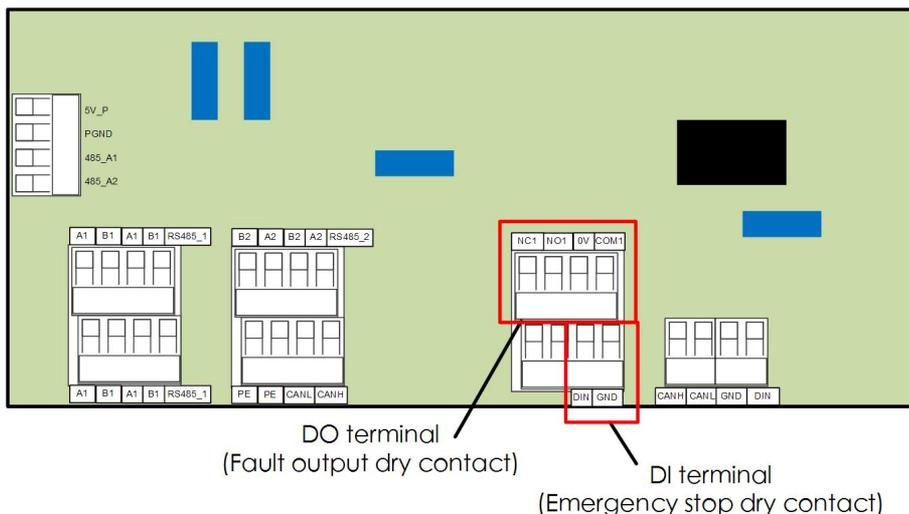
**DO terminal (fault output dry contact):** the relay can be set to fault alarm output, and user can configure it to be a normal open contact (COM&NO) or a normal close contact (COM&NC).
